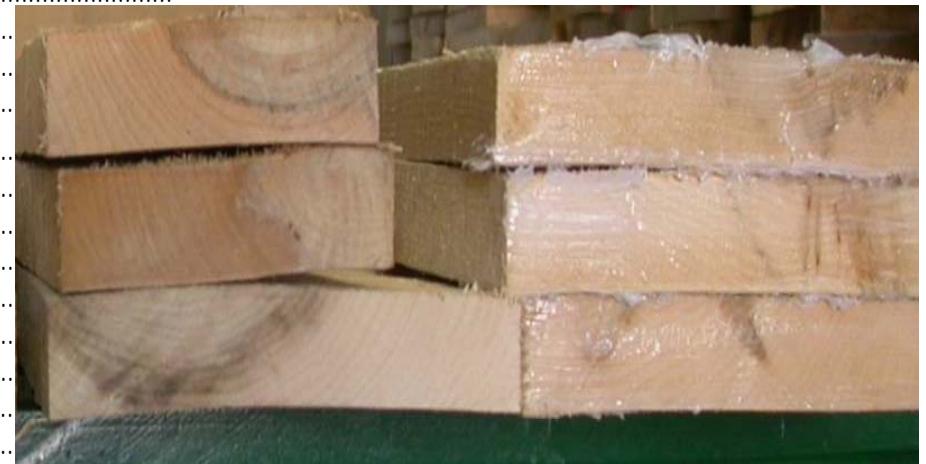
Figure 1 Boards protected with paraffin (left) and silicon (right) coatings against checking
