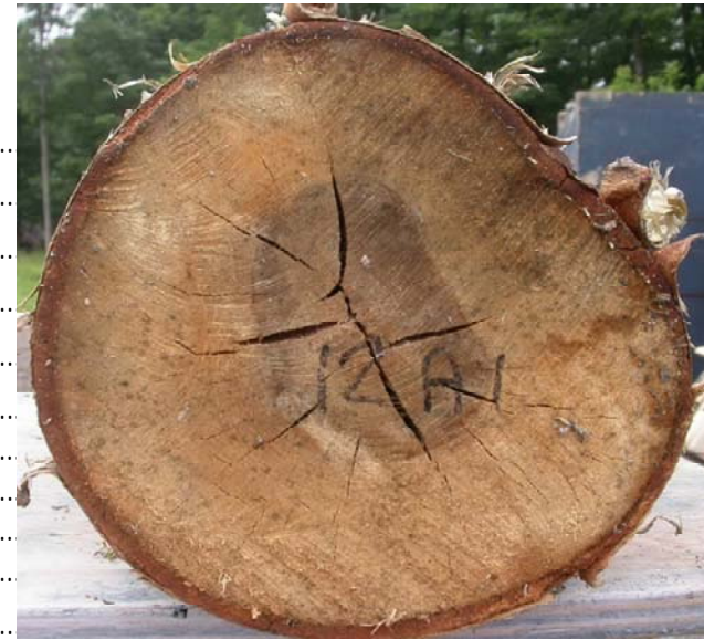
Figure 1 End checks occurred on a bark protected log
